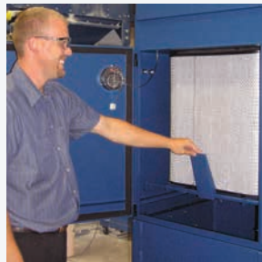
One pivot lever securely retains the primary filter element.
