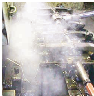
SMOKE Typical particle size: 0.07-1.2 micron
